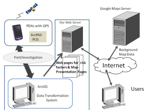
**Fig. 1. Conceptual Image of Our Location-based Service System**
