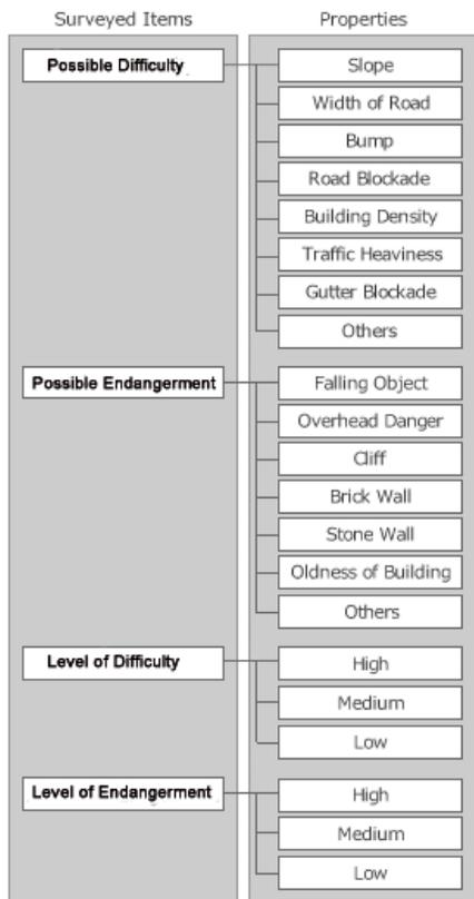
**Fig. 2. Data Architecture of Our Proposed System**
