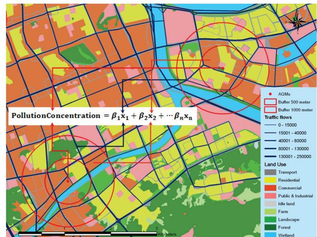
FIGURE 1 Air quality model based on traffic flows and land uses
