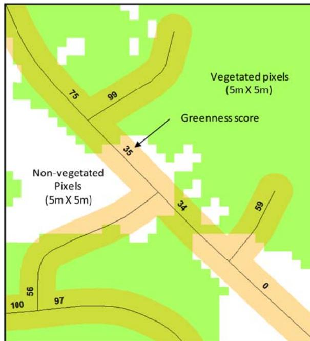
Figure 2: Calculation of the greenness score for each road segment based on the binary green image
