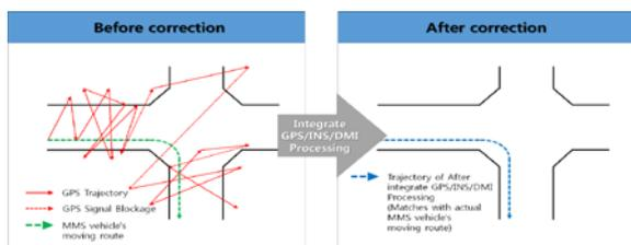
Fig. 3. Correction of MMS vehicle's location to integrate
