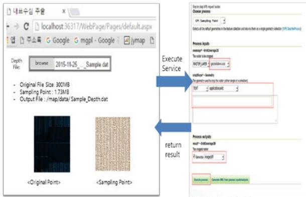
**Figure 3. Example of Representative Depth Extraction using WPS Service**
